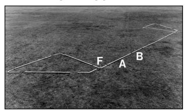
1. Lay out parts according to picture. Assemble top cross bar by sliding together pieces A, B, & F as shown.
